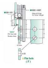
Complete G-Tech single door kit with wall mounts. Suitable for a single glass door mounted on a block or timber structure. Maximum door weight: 100kg.
