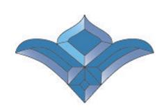
Regalead decorative glass bevels are designed primarily for the overlay market and are manufactured from 5mm float glass which is bevelled down to a 1.5  $\tilde{A}$  $\square$  1.8mm edge. These fine edges make the bevel pieces ideal for using with self adhesive lead but also suitable for customers working with traditional lead cames or copper foils.
