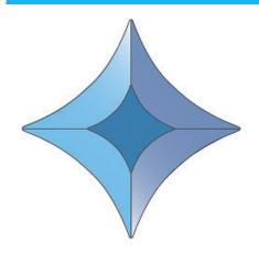
Regalead decorative glass bevels are designed primarily for the overlay market and are manufactured from 5mm float glass which is bevelled down to a 1.5  $\tilde{\Lambda}$  1.8mm edge. These fine edges make the bevel pieces ideal for using with self adhesive lead but also suitable for customers working with traditional lead cames or copper foils.
