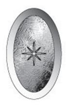
Regalead decorative glass bevels are designed primarily for the overlay market and are manufactured from 5mm float glass which is bevelled down to a 1.5  $\tilde{A}$  1.8mm edge. These fine edges make the bevel pieces ideal for using with self adhesive lead but also suitable for customers working with traditional lead cames or copper foils.
