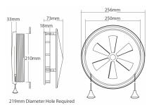
The Vent-A-Matic is a durable and effective in-glass ventilator that can solve most ventilation requirements. The SXL Rotary Vent is equipped with a diffusing rotor which helps to prevent severe drought and improve fresh air distribution within the room. The rotor also continues to operate whilst under its own inertia, even when air pressure on each side has been equalised.
