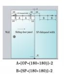
OP=Overpanel width SP=Sidepanel width DP=Door panel width
