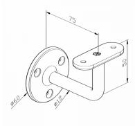
• 304 grade stainless steel wall to handrail bracket flat saddle.
