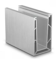
Ideal small and slim system for mounting on to the side of a parapet wall to increase the height of it up to 1100mm high and achieve suitable barrier loads of up to 0.74kn with the correct glass selection. Can also be used to fix to the side of a full height wall to act as an additional windbreak without losing the views that a wall would result in.
