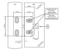
• The MagnaLatch Side Pull Model is an inexpensive, magnetic gate latch that offers simple, effective latching for swimming pool and other glass gates.
