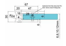
$\bullet$  A 63mm x 45mm D shaped clamp. Suitable for mounting to a 48mm diameter post.
