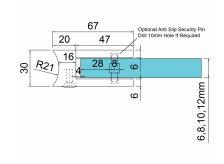
$\bullet$  A 63mm x 45mm D shaped clamp. Suitable for mounting to a 42mm diameter post.
