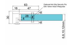
$\bullet$  A 63mm x 45mm D shaped clamp. Suitable for mounting on a flat surface.
