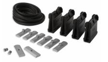
• Included are the clamp bars, which sit into the top mould of the clamps and the clamp bolts, which screw into the bars and are then undone to hold the glass in place. These are undone and tightened each side allowing the glass to be aligned. 6 metres of gasket to suit your glass thickness is also included.
