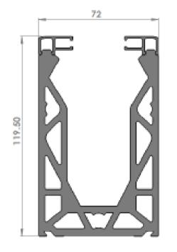
Figure B3 Posi-Glaze Dimensions With Top Seal
