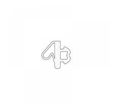
• Gaskets used where the glass door meets the aluminium rebate of the door frame profile ensuring a soft close and reduced noise and air movement.
