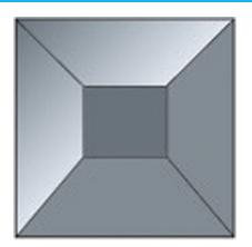
Regalead decorative glass bevels are designed primarily for the overlay market and are manufactured from 5mm float glass which is bevelled down to a 1.5  $\tilde{A}$  1.8mm edge. These fine edges make the bevel pieces ideal for using with self adhesive lead but also suitable for customers working with traditional lead cames or copper foils.
