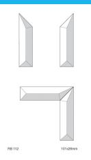
• Regalead decorative glass bevels are designed primarily for the overlay market and are manufactured from 5mm float glass which is bevelled down to a 1.5 - 1.8mm edge.
