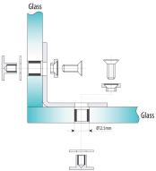
$\bullet$  It consists of turned articles and screws in stainless steel AISI 316L to fix the angle bracket with L-junction between glass and glass.
