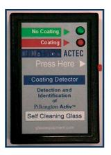
• This device detects the tin bath side of float glass.
