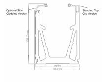
• The Heavy-Duty Commercialised and Fully Adjustable 3Kn Frameless Balustrade System.
