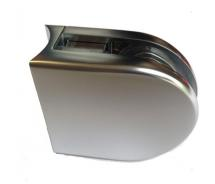
Special Clearance Sale Item. Diecast aluminium clamp in a satin silver finish. Suitable for mounting to a  $42\,\mathrm{mm}$  diameter post and for 6 -  $8\,\mathrm{mm}$  thick glass. Internal use.
