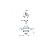
• Drilled glass shelf support for use with the rod system.
